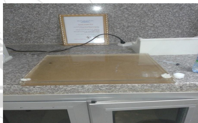
Figure 2: shows the back part simulates the liquid flood phantom made of Perspex (42×42×1 cm) and has orifice 0.5 cm to be fill with a liquid radioactive material
