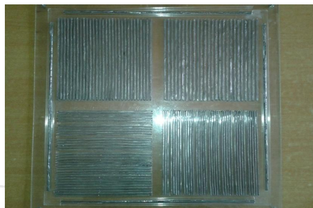
Figure 1: shows the frontal part of the phantom made of Perspex (42×42×10 cm) that simulates the four quadrant bars phantom each one was 20×20 cm
